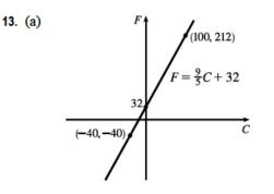
(b) The slope of <sup>9</sup>/<sub>5</sub> means that F increases <sup>9</sup>/<sub>5</sub> degrees for each increase of 1°C. (Equivalently, F increases by 9 when C increases by 5 and F decreases by 9 when C decreases by 5.) The F-intercept of 32 is the Fahrenheit temperature corresponding to a Celsius temperature of 0.
